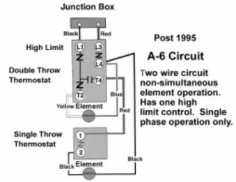
**A-6 Circuit** - Standard on dual element water heaters non-simultaneous/interlocked operation.
